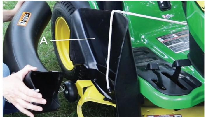
2. Slide the metal rod (B) on the front of the Deck Chute (C) through the hole in the front gauge wheel and attach the bungee cord (D) on the front of the Deck Chute support on the right side of the mower deck.
